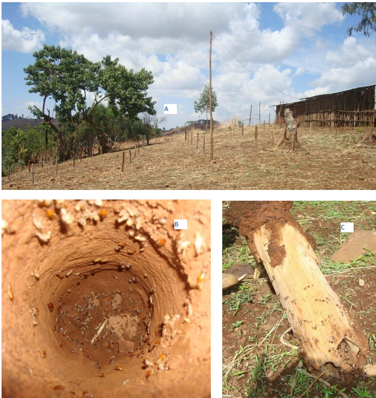
Figure 2. Wooden construction material experiment layout (A) and termite infested planting hole after removing the wooden sticks (B) and termite damaged wooden sticks (C).
