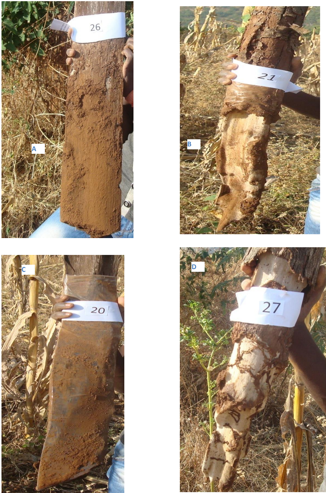
Figure 1. Chlorpyrifos 48% E. C. treated bare planted (A), untreated but polyethylene bag covered (B), chlorpyrifos 48% E. C. treated and polyethelene bag covered (C) and lastly untreated and bare planted (D) wooden sticks.
